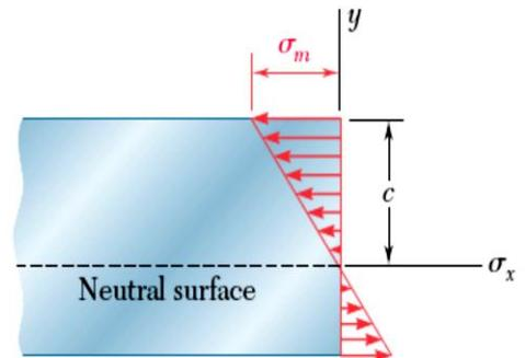
Fig. 5 Bending stresses.
