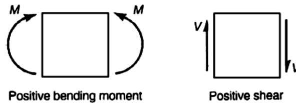
Figure 9.12 Sign convention for bending moment and shear
