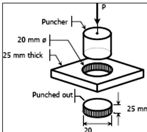
The resisting area is the shaded area along the perimeter and the shear force  $V$  is equal to the punching force  $P$ .
