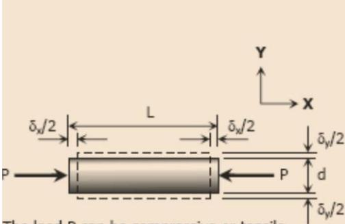
The load  $P$  can be compressive or tensile
