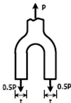
For shearing of rivets (double shear)
