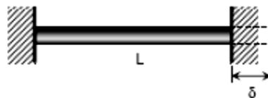
deformation due to temperature changes;
