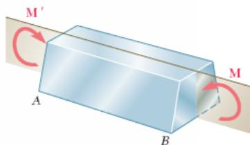
Fig.1 Member in pure bending.
