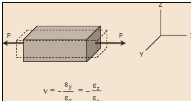
where  $\epsilon_x$  is strain in the x-direction and  $\epsilon_y$  and  $\epsilon_z$  are the strains in the perpendicular direction. The negative sign indicates a decrease in the transverse dimension when  $\epsilon_x$  is positive.
