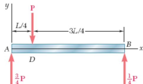
Fig. 9.27 Free-body diagram for beam of Fig. 9.16.
