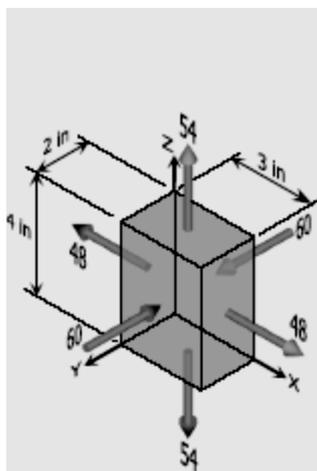
For triaxial deformation (tensile triaxial stresses):
