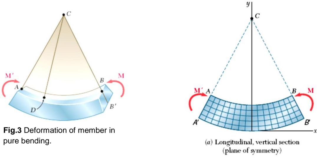
Fig.3 Deformation of member in pure bending.
