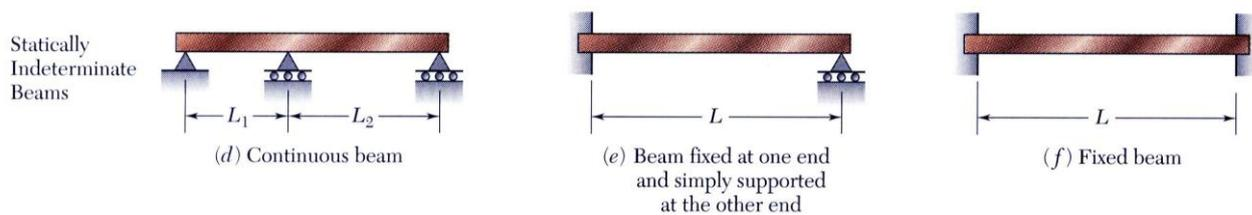
**The degree of indeterminacy** is taken as the difference between the number of reactions to the number of equations in static equilibrium that can be applied. In the case of the propped beam shown, there are three reactions ( $R_1$ ,  $R_2$ , and  $M$ ) while only two equations ( $\Sigma M = 0$  and  $\Sigma F_v = 0$ ) can be applied, thus the beam is indeterminate to the first degree ( $3 - 2 = 1$ ).
