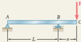
The overhanging steel beam *ABC* carries a concentrated load *P* at end *C*. For portion *AB* of the beam, (a) derive the equation of the elastic curve, (b) determine the maximum deflection, (c) evaluate  $y_{\max}$  for the following data:
