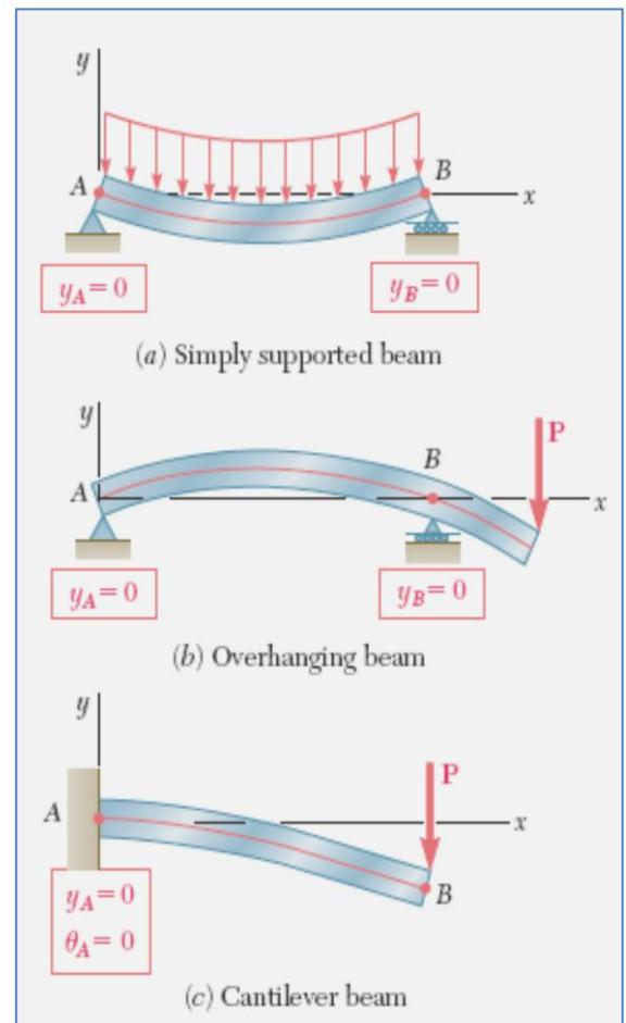
The cantilever beam  $AB$  is of uniform cross section and carries a load  $P$  at its free end  $A$  (Fig. 9.9). Determine the equation of the elastic curve and the deflection and slope at  $A$ .
