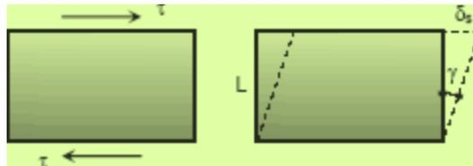
The change in angle at the corner of an original rectangular element is called the **Shear Strain**( $\gamma$ ) and is expressed as:
