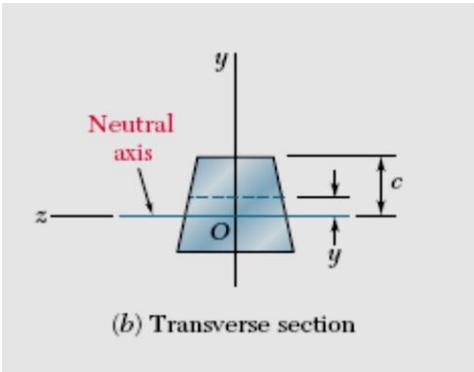
Fig. 4 Deformation with Respect to Neutral Axis
