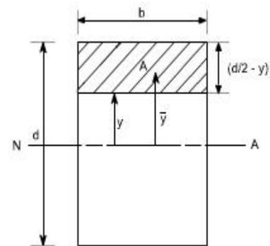
This shows that there is a parabolic distribution of shear stress with  $y$ .
