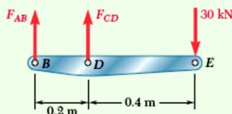
Fig. 1 Free-body diagram of rigid bar  $BDE$ .
