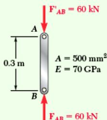
Fig. 2 Free-body diagram of two-force member  $AB$ .
