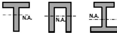
The proportioning of these sections is such that the ratio of the distance of the neutral axis from the outermost fibers in tension and in compression is the same as the ratio of the allowable stresses in tension and in compression. Thus, the allowable stresses are reached simultaneously.
