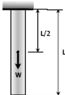
The weight will act at the center of gravity of the bar:
