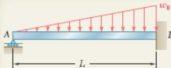
For the uniform beam AB, (a) determine the reaction at A, (b) derive the equation of the elastic curve, (c) determine the slope at A. (Note that the beam is statically indeterminate to the first degree.)
