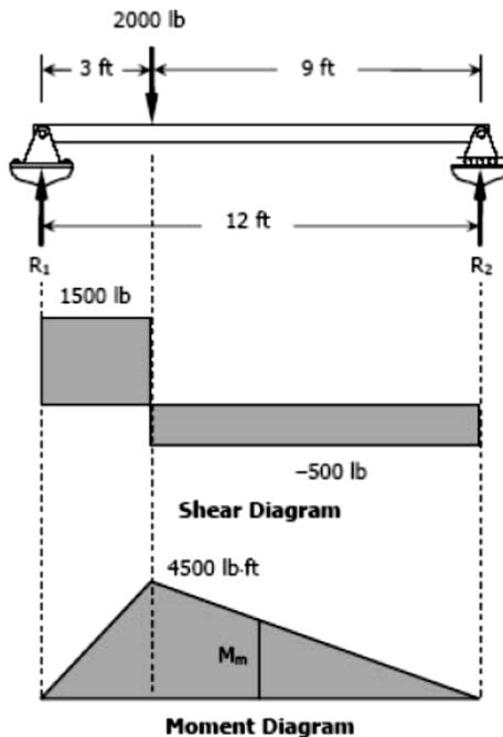
$$\begin{aligned}\Sigma M_{R2} &= 0 \\ 12R_1 &= 9(2000) \\ R_1 &= 1500 \text{ lb}\end{aligned}$$
