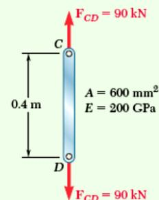
Fig. 3 Free-body diagram of two-force member  $CD$ .
