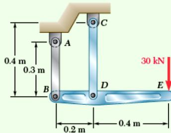
The rigid bar  $BDE$  is supported by two links  $AB$  and  $CD$ . Link  $AB$  is made of aluminum ( $E = 70$  GPa) and has a cross-sectional area of  $500 \text{ mm}^2$ . Link  $CD$  is made of steel ( $E = 200$  GPa) and has a cross-sectional area of  $600 \text{ mm}^2$ . For the  $30\text{-kN}$  force shown, determine the deflection ( $a$ ) of  $B$ , ( $b$ ) of  $D$ , and ( $c$ ) of  $E$ .
