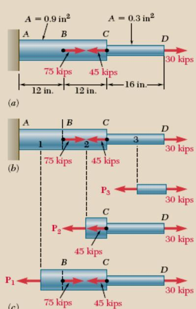
**Fig. 2.19** (a) Axially-loaded rod. (b) Rod divided into three sections. (c) Three sectioned free-body diagrams with internal resultant forces  $P_1$ ,  $P_2$ , and  $P_3$ .
