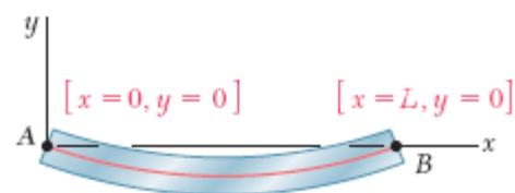
Fig. 9.28 Boundary conditions for beam of Fig. 9.16.
