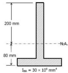
$$\begin{aligned} M_t &= \frac{40(30 \times 10^6)}{80} \\ &= 15\,000\,000 \text{ N}\cdot\text{mm} \\ &= 15 \text{ kN}\cdot\text{mm} \end{aligned}$$
