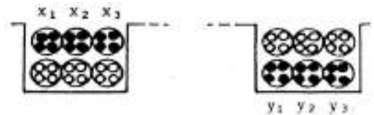
Fig. 3.5 Two-layer winding with 3 coil sides per slot per layer.
